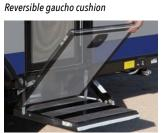
The E-Z Swing Stepper Door with hydraulic assist, operates in seconds and provides the largest, most stable step platform in the industry.
