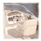
The helmsman oversees an instrument panel with custom backlit instrumentation. Power tilt and trim and a tilt steering wheel with power steering make piloting easy and enjoyable.
