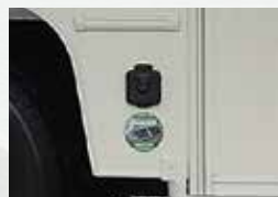
Solar panel plug-in connection. Solar-ready Connection (standard)
