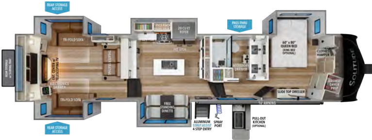
376RD U 1 V 1 W 1 HITCH 1 GVWR LENGTH 2 HEIGHT 3 CAPACITY 15,400 3,100 19,000 42' 6" 13' 5" 83 106 53
