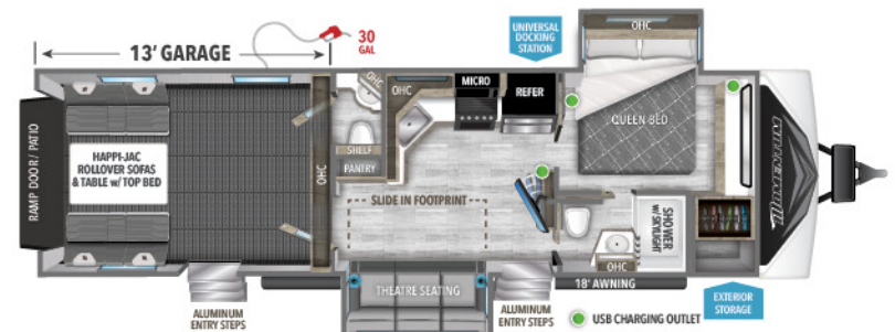
31G 13' GARAGE UVW' EMPTY HITCH' GVWR LENGTH' HEIGHT CAPACITY 8,975 1,600 13,000 35' 11" 12' 4" 96 37 39 37* * 1/2 BATH DOUBLES AS BLACK/GREY
