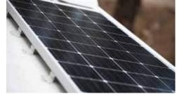
Roof Mounted 190W Solar Panel (1 or 2) assists in keeping your battery(s) charged.
