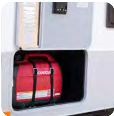
Portable Generator Storage Compartment W/Tie-Downs
