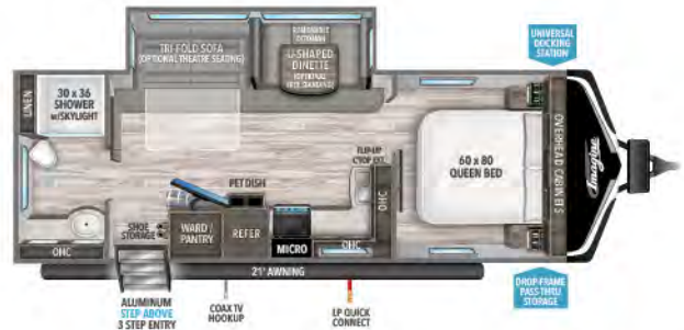
2600RB UVW 1 5,795 HITCH 1 594 LENGTH 2 29' 8" HEIGHT 11' 1" CAPACITY 52 82 45
