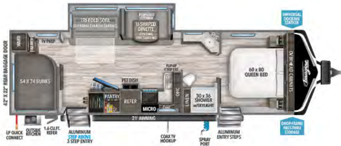
2910BH UVW 1 7,087 HITCH 1 720 LENGTH 2 33' 11" HEIGHT 11' CAPACITY 52 90 45
