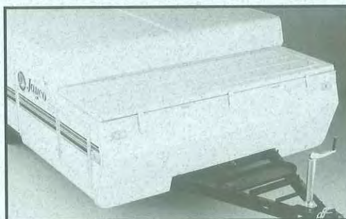
A full-width ABS door provides easy outside access to the storage trunk when your fold-down is closed for travel.
