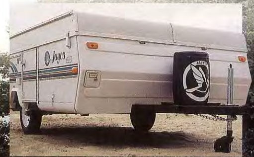
Front and Rear End Caps are made of good-looking, hard-wearing, dent-resistant ABS
