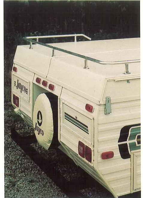
The new Jayco fold-down roof rack is an option that can increase your luggage carrying capabilities.
