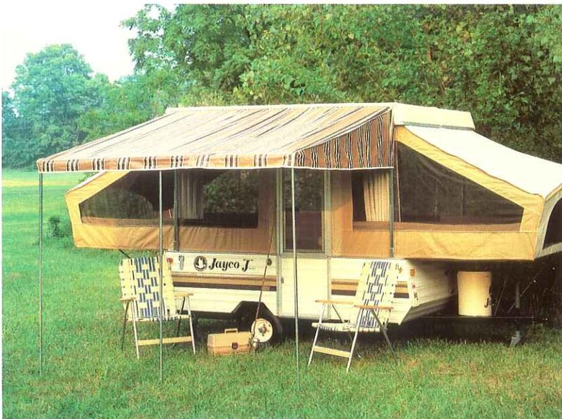
Here, our "J" Series model 1008 features our optional canopy. Its unique design incorporates free-standing spring-loaded support poles to keep the fabric extra-taut. The Jayco canopy is easy to install on any model of "J" Series fold-down.
