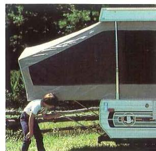
By easily inserting support bars under the end bunks, extra stability and rigidity is imparted to these wings. That's all there is to it!
