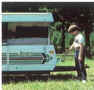
Turn the crank, and the roof begins to rise . . . almost without effort. A brake mechanism reduces the danger of free-fall. And there are no awkward arms to contend with.
