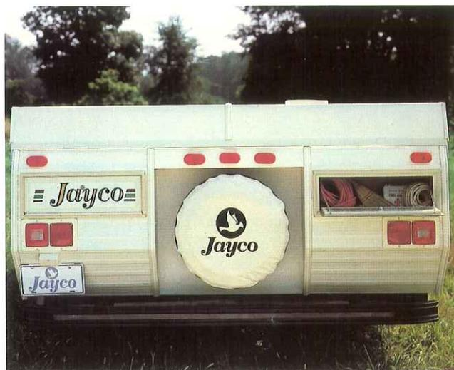
The spare tire is recessed so that the bumper is the most rearward point on the camper for safety purposes. The back lights are flush-mounted for safety and smooth appearance. And Jayco makes maximum use of every inch of the fold-down with lockable rear storage compartments.
