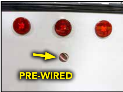
Backup Camera Prep
