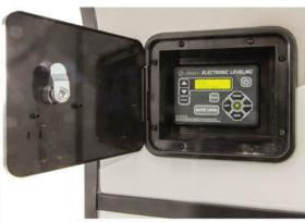
Six point hydraulic auto leveling is faster, stronger, guieter, and makes short work of leveling your coach so you can get to relaxing. We mount the control panel in a compartment on the off-door side by the front jacks.
