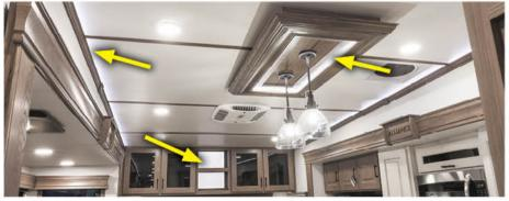
Alliance features LED accent lighting built into the crown molding, kitchen soffit, kitchen sink, select cabinet backs, and even the bathroom mirror. Create an appealing indirect glow that looks great day or night. Pendants with heavy glass globes swing and rip out of the ceiling when the trailer makes an abrupt stop. Our lightweight pendant lights don't have the mass and inertia to get moving and rip out at abrupt stops.
