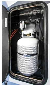
Extend your RV stay a little longer with 60 pounds of LP in two 30 pound tanks, located on both sides of the coach for even weight distribution and equipped with an auto changeover valve. For those wanting even more, dual 40
