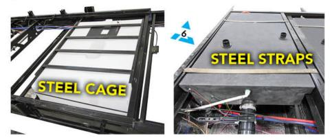
Our fresh tanks are encased in a robust steel cage. Waste tanks are molded to rest on full length steel Z rails and secured with steel straps to prevent shifting in transit.
